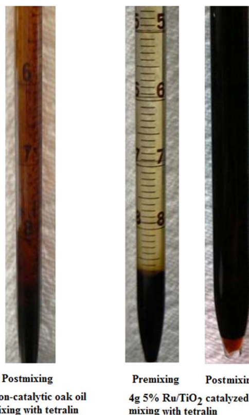
Figure 8. Compatibility test with tetralin for oak blank and catalytic vapor-upgrading liquid products.
